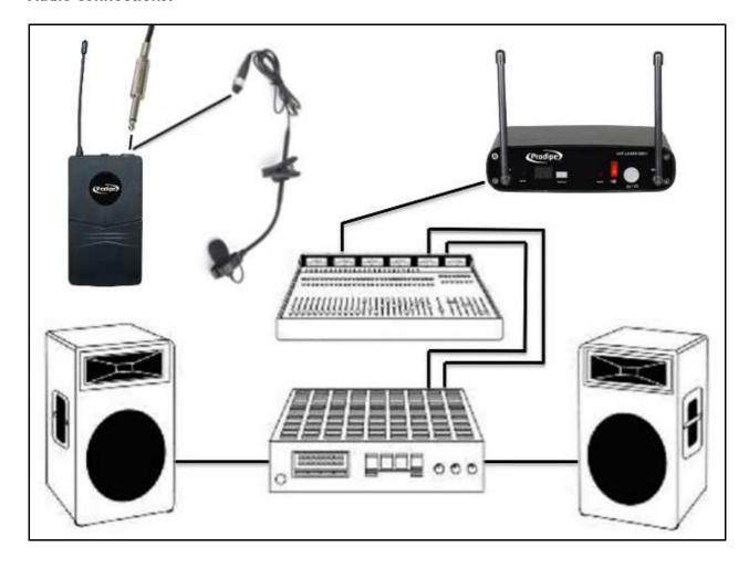
Connect the guitar/bass guitar active extension cable with jack or the Prodipe Series 21 mic mini XLR to the bodypack transmitter (UHF21).
