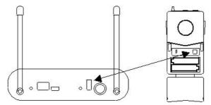
Channel selection is automatic. Ensure that the bodypack infrared sensor is in line with the receiver (about 10cm distance). Press quickly on the receiver SCAN IR button and the synchronisation will start automatically. Once the automatic scan has finished, the channel will be displayed on the channel display screen and the RF reception indicator light will come on.
